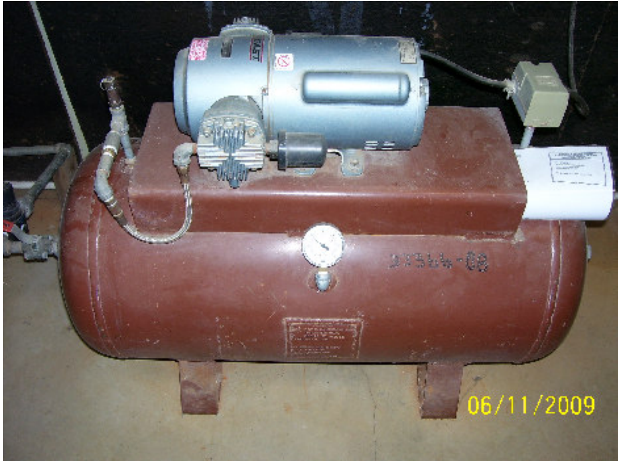
Oiless Air Compressor w/30 Gal Tank 120 volts 3/4 HP
